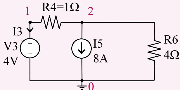
$$\begin{aligned} \text{Ek Denk: } V_1 &= V_3 \\ V_1 &= 4V \end{aligned}$$
