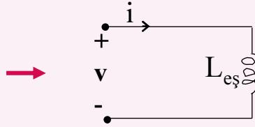
$$i(t) = \frac{1}{L_1} \int_0^t v dt + I_1(0) + \frac{1}{L_2} \int_0^t v dt + I_2(0)$$
