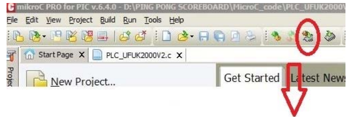
Upload the code to the PLC using one button
