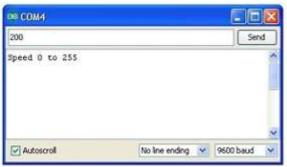
In the 'loop' function, the command 'Serial.parseInt' is used to read the number entered as text in the Serial Monitor and convert it into an 'int'. You can type any number here. The 'if' statement in the next line simply does an analog write with this number, if the number is between 0 and 255.
